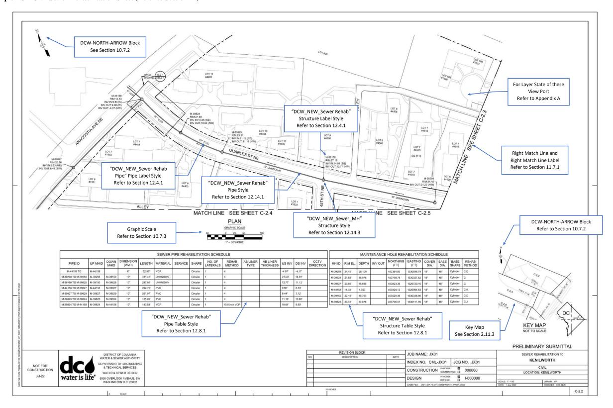
Example – S – Civil Sewer Rehabilitation Sheet (Refer to Section 12.9.4)
